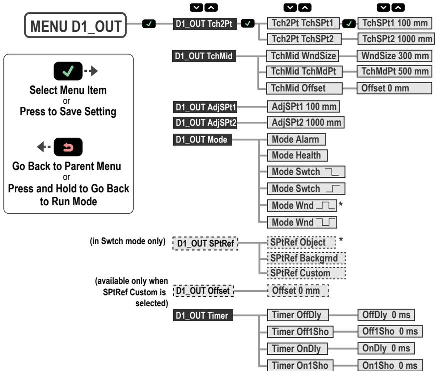
Figure 16. Discrete 1 Output Menu Map (Discrete 2 is identical)
