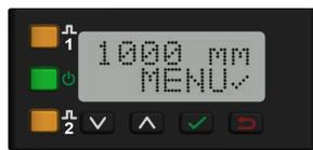
Figure 2. LE550 Display in Run Mode
