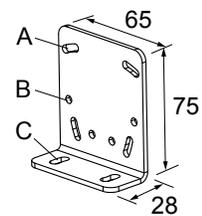
Hole size: A =  $\varnothing$  4.5 with 20° adjustability, B =  $\varnothing$  4.5, C =  $\varnothing$  5.7 with 20° adjustability
