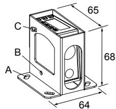
Hole size: A =  $\varnothing$  5 with 20° adjustability, B =  $\varnothing$  4.5, C =  $\varnothing$  4.5 with 10° adjustability
