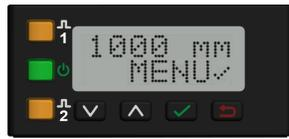
Figure 22. LE550 Normal Display Orientation
