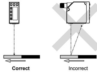
Figure 9. Orientation for a color or luster difference
