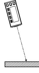
Figure 10. Orientation for a highly reflective target
