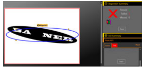
Figure 200. Bad Part—Missing Letter
