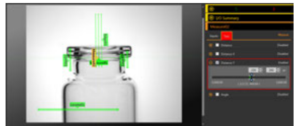
Figure 177. Bad Part—Missing Stopper
