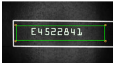
Figure 103. Light Date/Lot Code on a Dark Background
