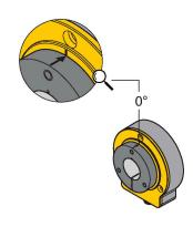
The extensive range of mounting accessories enables easy adaptation to many different shaft diameters. Due to the measuring principle, which is based on the functional principle of an RLC coupling, the encoder is immune to magnetized ferrous chips and other interferences. As a result, there are few possible causes of error during mounting. The adjacent figures show the simple installation of the two separate units: the sensor element and the positioning element: Mounting option A:
