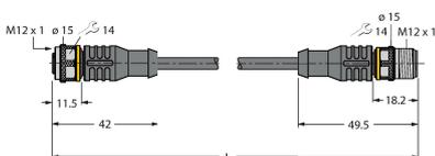
Extension cable, M12 female connector, straight, 4-pin to M12 male connector, straight, 4-pin; cable length: 2 m, jacket material: PUR, black; cULus approval
