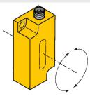
Adjusting the measuring range via TX1-Q20L60 teach adaptor
